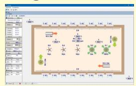
The adjustment of multi-point characteristics of the inlets opening in the function of ventilation efficiency- optimisation of the underpressure.
